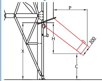
**Important:** The Low level side discharge silo has a clearance of 1.7m under the cone. Please ensure that the correct chute is specified from the options below to suit the discharge target. i.e. bucket or trailer.
